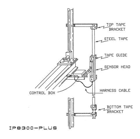
Figure 3. Complete Unit With Top And Bottom Brackets
