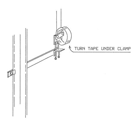
Figure 2. Bottom Tape Bracket
