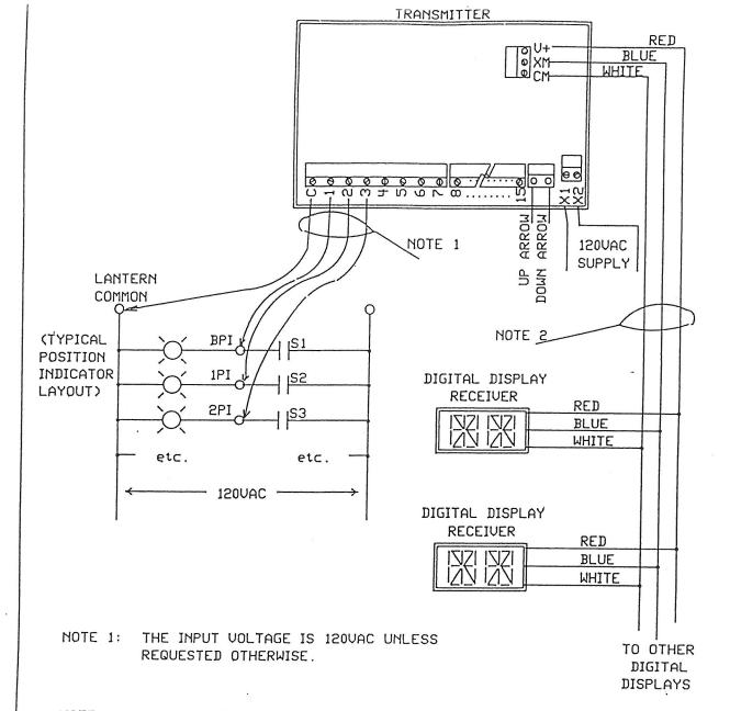
NOTE 2: THE SIZE OF THE THREE WIRES TO THE RECEIVERS WILL DEPEND UPON THE DISTANCE AND THE NUMBER OF RECEIVERS.
